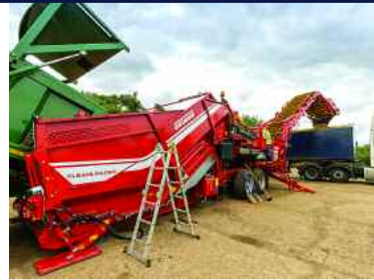
The CleanLoader has the capability to deliver an output of up to 120t/hour depending on soil type, crop, and conditions.
