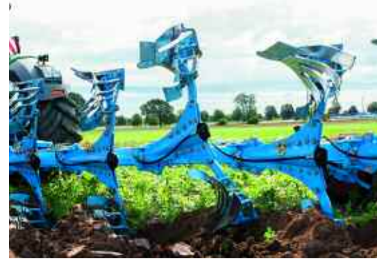
Users of Lemken's Juwel, Diamant and Titan ploughs can now also benefit from the newly launched OptiStone automatic overload protection.
