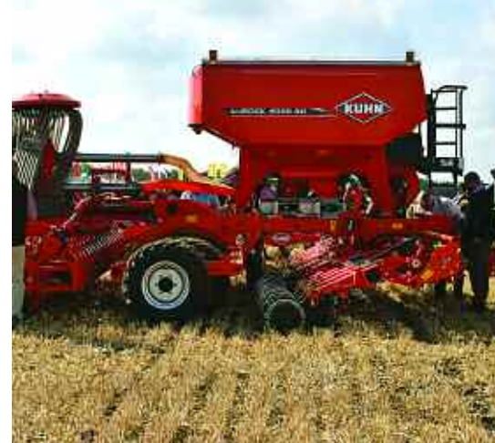
Kuhn's Aurock 6m 6000 RC drill features dual metering and a 5000-litre capacity split hopper.
