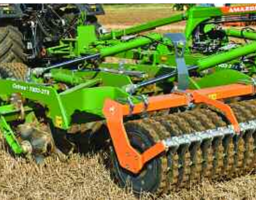
The stubble arena provided a stage for an array of cultivation methods from ploughs to low disturbance options and among them was Amazone's 7m Catros with cross cutter discs.
