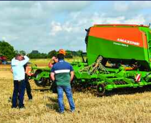
The Cayena tine coultter seed drill has been designed for high-speed sowing on hard, dry and stony soils with or without prior soil tillage.
