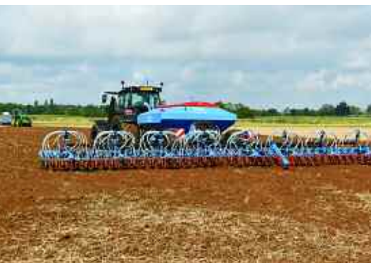
The Solitair 12 trailed pneumatic seed drill is available in working widths of 8m to 12m.
