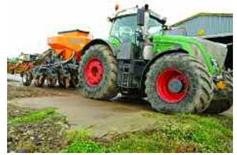
Direct drilling wheat into grass with the Mzuri drill is helping to preserve soil structure, compared with a combi drill.
