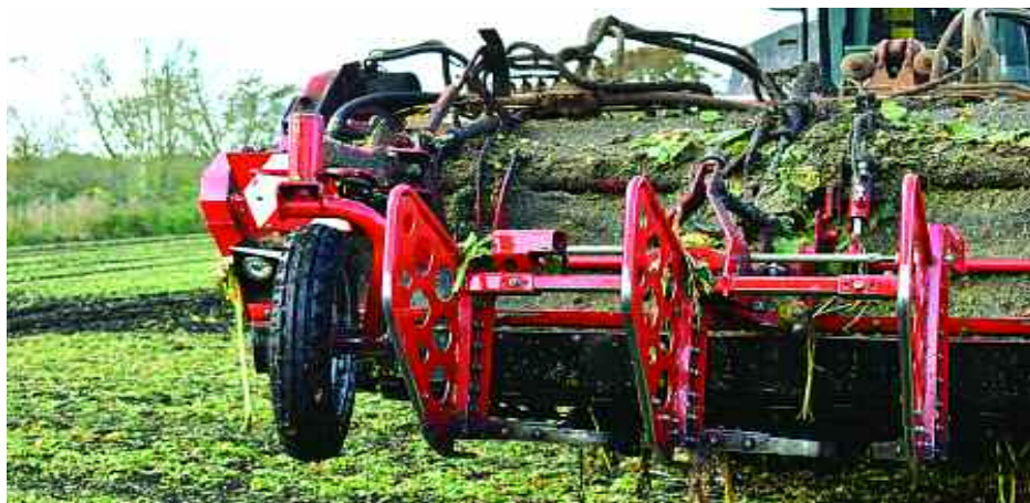
The Rexor is fitted with a variable topper that enables side discharge of beet tops.
