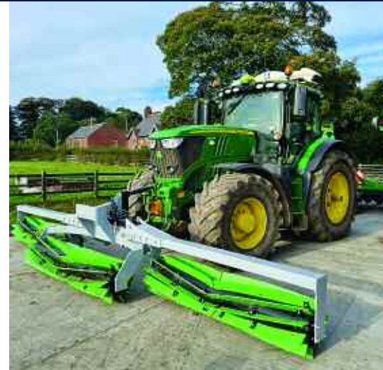
Especially suited to organic systems, the CombeCut is a mechanical weeder which can be attached to a tractor.
