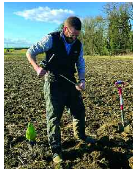
The Agrii team has developed programmes to help determine soil condition using tools such as penetrometer tests.
