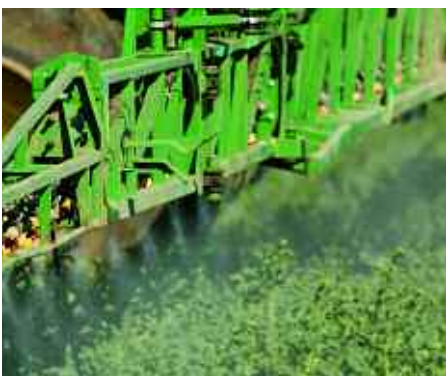
Pulse width modulation has helped eliminate both over and underdosing of chemistry on farm.
