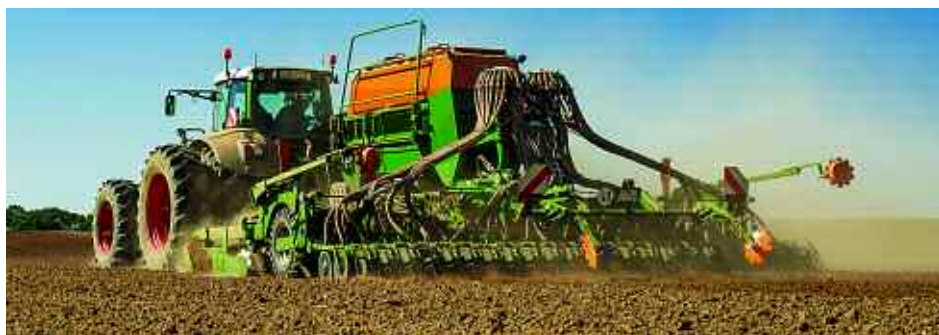
Amazone's Cirrus 6003-2C can sow crops directly into a standing catch crop.
