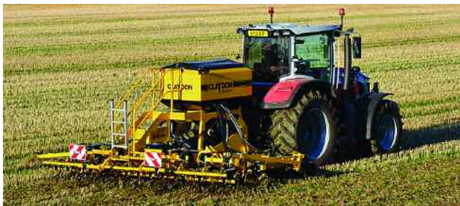
Claydon's Evolution direct strip till drills offer growers the opportunity to drill seed and fertiliser together.
