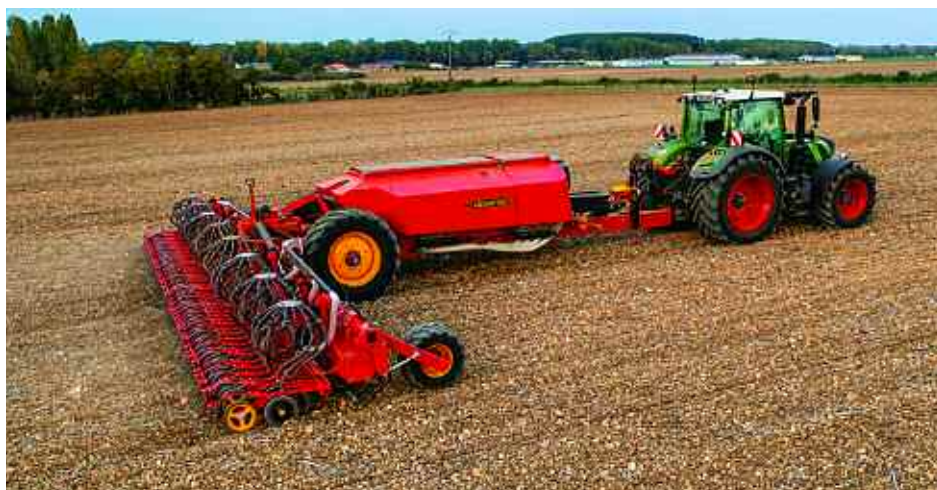
Väderstad's Inspire is a high-capacity double disc seed coultter drill that's due to be available from the end of 2022.
