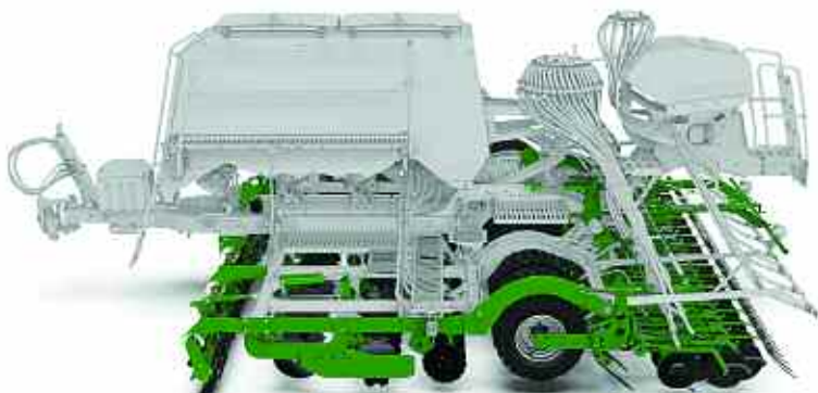
The knife-roller is a new front tool for Amazone's Cirrus 6003-2 min-till drill.
