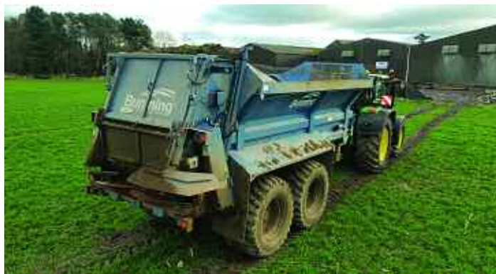
The elevated height of the spreading body helps the rear discs comfortably spread material to 24m.
