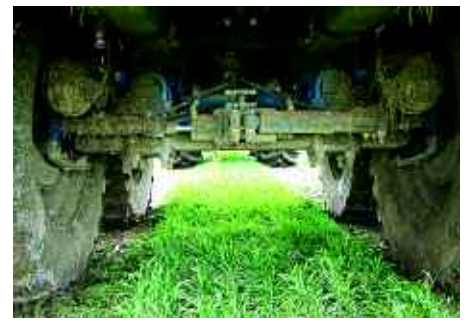
A rear steering axle has helped limit crop damage when turning.
