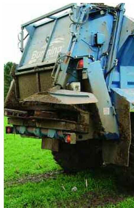
The rear door has five settings for drop point adjustment depending on the material.
