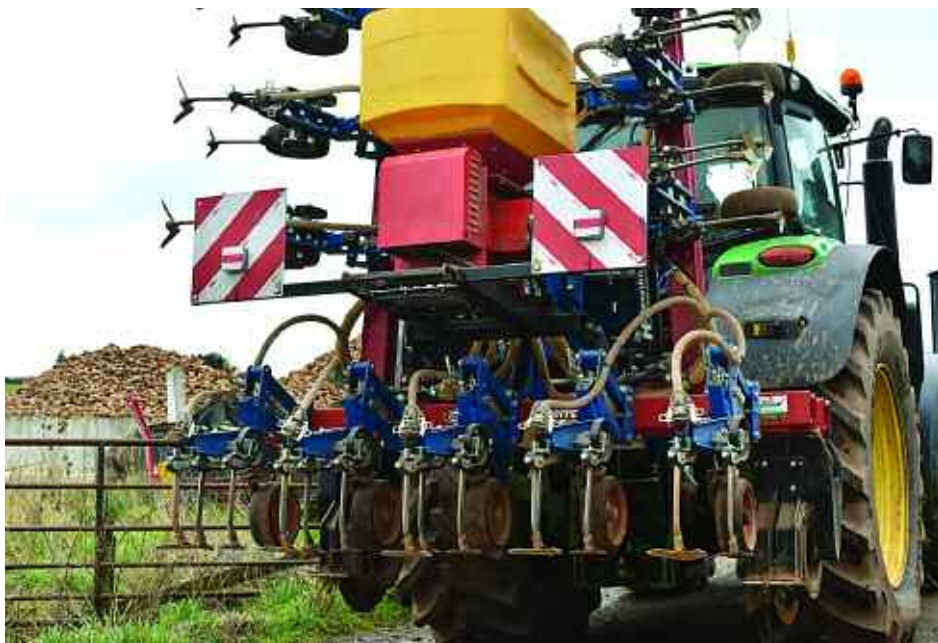
A 12-row, 6m inter-row cultivator, set at 50cm spacings, arrived at Gillow Farm last spring.
