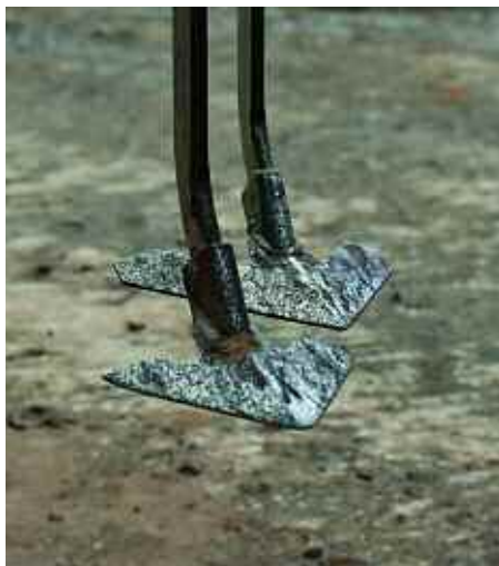
The hoe works between rows of growing crops to cut off weeds just below the surface via vibro-tines with duck foot shares.
