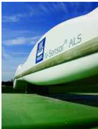
Information from the N-Sensor can help assess how much N the crop contains in real-time so rates can be adjusted accordingly.
