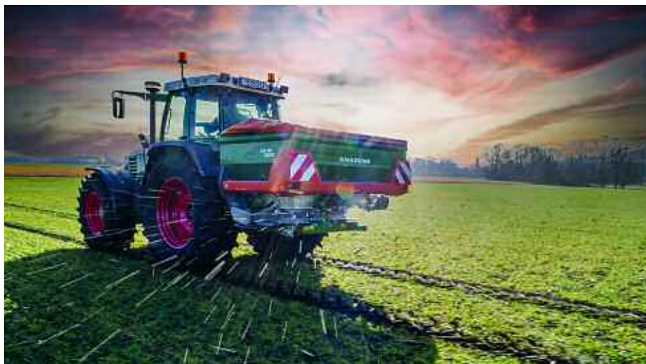
EasySet 2 ensures a consistently precise spread pattern and increases work rates by being able to vary the forward speed.
