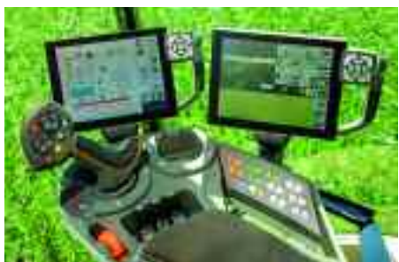
Inside the cab, the Rogator 600 series benefits from ISOBUS as well as some of Fendt's in-house features including the OptiControl leaver and the Optiflow control panel.
