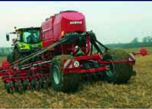
The Horsch Avatar features 16.7cm-spaced single disc coulters arranged over two rows, with 33.4cm clearance per row, to handle high trash levels.
