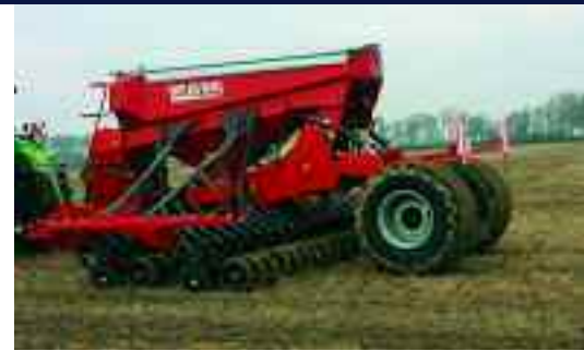
While most smaller mounted direct drills are of the tine coulters type, Weaving offers its GD double disc coulters machines right down to 3m mounted sizes.
