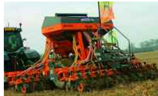
Ma/Ag's Sicura SSP, from Ryetec, features floating disc coulters with individual pressure adjustment and depth control, each floating on a parallel linkage.
