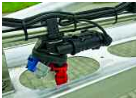
Danny Milazzo's Rogator benefits from individual section control as well as the 2+2 DualSelect nozzle select tool.
