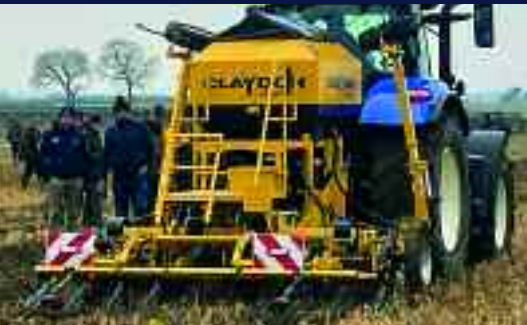
Claydon's Hybrid can be configured in multiple ways: the standard opener, with leading tine or single/double disc openers, and single or twine seeding tine options.
