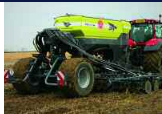
Sky's EasyDrill HD features a 'Tandem' seeding arrangement, said to aid depth stability when large stones and clods are encountered.
