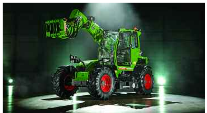
Fendt's new Cargo T740 features TopViewCab capability, meaning the cab can be raised to different levels.
