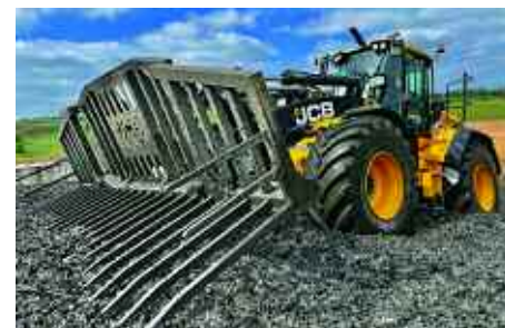
The engine of JCB's new wheeled loader produces 282hp with 1200Nm of torque, providing a power to weight ratio of 14hp/t.
