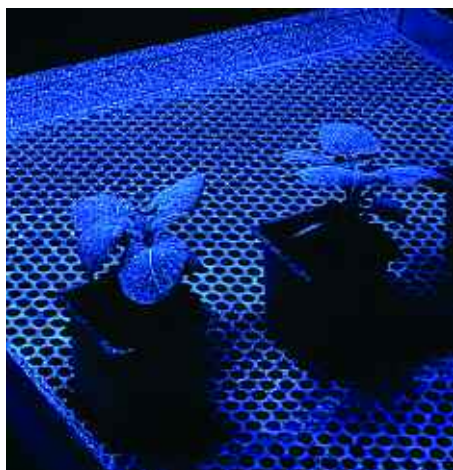
A UV light is used to demonstrate spray pattern and coverage.
