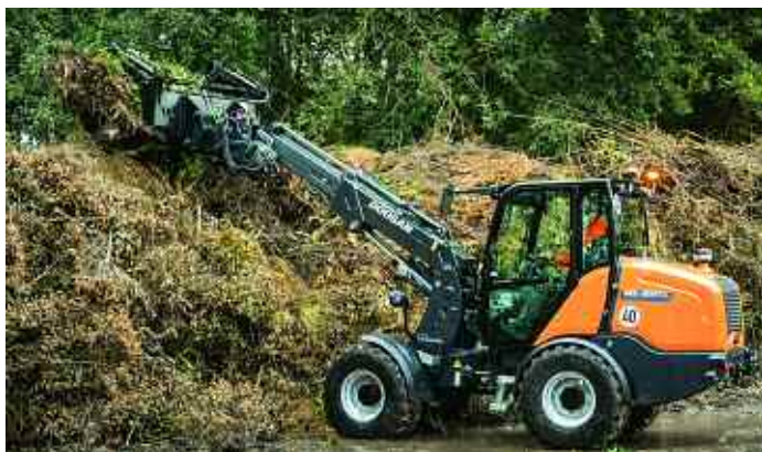
The new compact wheel loaders have Stage V engines, hydrostatic 4WD, 100% differential lock on both axles and high lift capacity.
