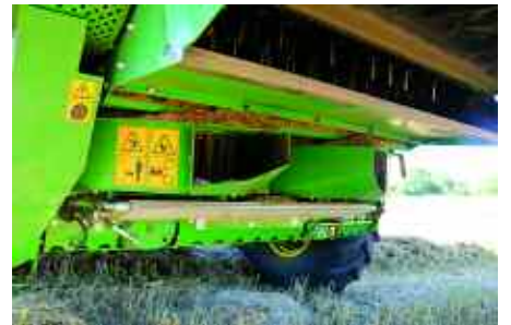
The rotors receive the chaff and weed seed from the back of the sieving shoe and move it through a series of rotating and stationary tungsten carbide-coated columns.
