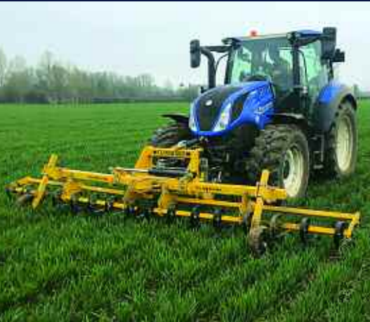
The 4.8m Claydon TerraBlade operating in a crop of wheat at Clattercote Priory, providing mechanical weed control.
