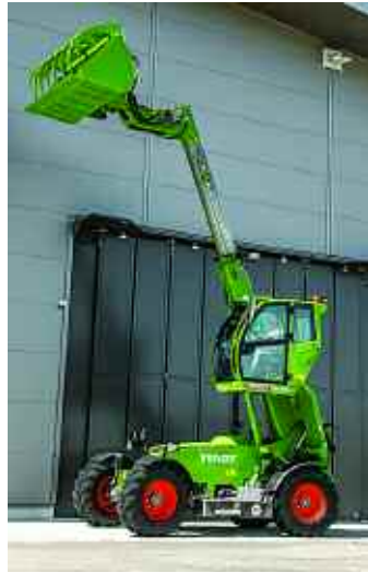
The Cargo T740 has a four-cylinder Cummins engine, producing 136hp which is able to achieve 20km/h as standard.
