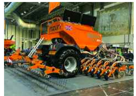
The new iPASS from Mzuri features a 5000-litre pressurised tank to meter and convey high application rates for seed and fertiliser.
