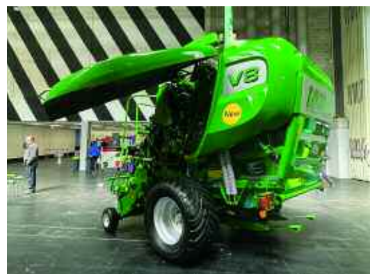
The new V8 range from McHale features its largest variable chamber balers, capable of producing a bale up to 1.9m in diameter.
