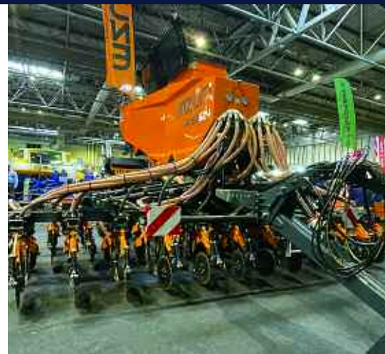
The iPASS has been designed to be capable of drilling into a range of surface types, including cover crops, stubble, grassland and cultivated ground.
