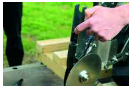
The metering disc (left) is 3D-printed and can be made to order. Seed drops down to the shoe (right) where a gate opens to let it into the soil at precisely the right moment.
