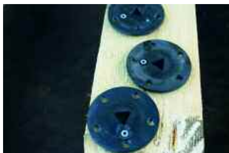
The metering disc (left) is 3D-printed and can be made to order. Seed drops down to the shoe (right) where a gate opens to let it into the soil at precisely the right moment.
