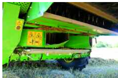
The rotors receive the chaff and weed seed from the back of the sieving shoe and move it through a series of rotating and stationary tungsten carbide-coated columns.
