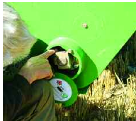
Andy Young (left) finds putting the unit in and out of work relatively quick and simple, with a rather neat clutch disengaging the drive (right).
