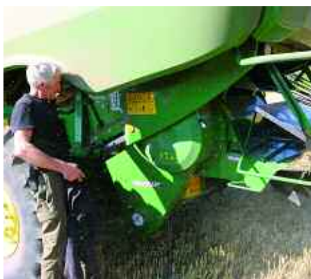
Andy Young (left) finds putting the unit in and out of work relatively quick and simple, with a rather neat clutch disengaging the drive (right).
