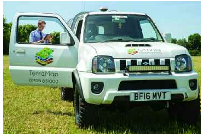
The TerraMap methodology collects data in two steps; scanning by driving a lightweight all-terrain vehicle fitted with the sensor over a field, and then taking soil samples to allow for each scan to be used to create the individual map layers.
