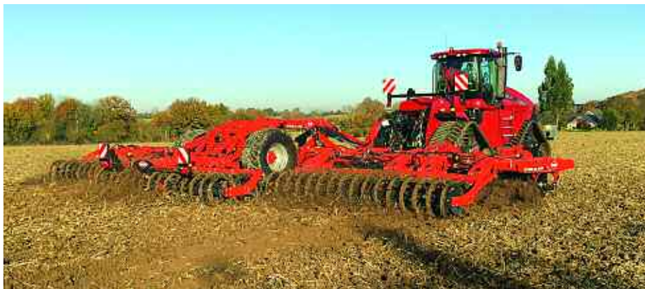
Kuhn's Optimizer XL is its first 12m machine to feature its Steady Control system which aims to maintain a uniform working depth.
