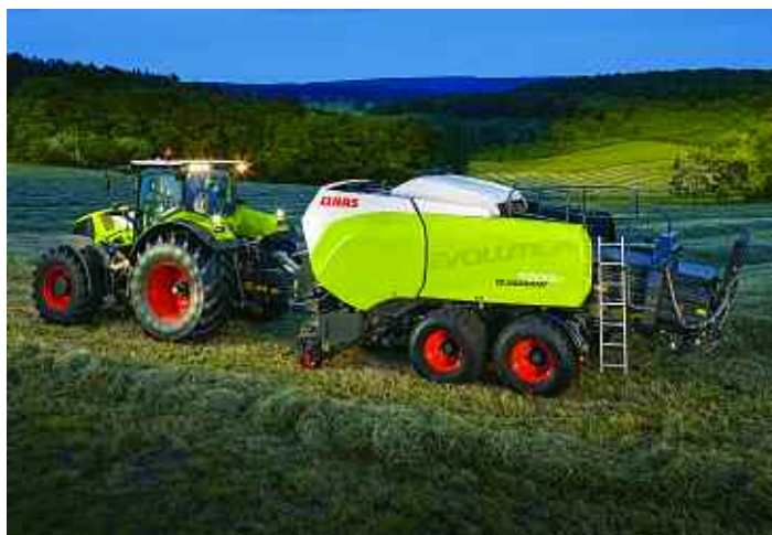
Claas has reengineered its Quadrant square baler with a new HD pick-up with two cam tracks to increase output and durability.
