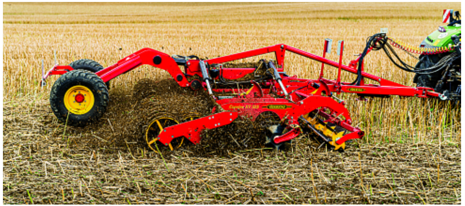
Väderstad's Carrier XT disc cultivator is designed for high-speed primary tillage and seedbed preparation.
