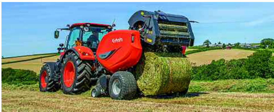
Kubota's new high capacity BF3500 fixed chamber baler has been developed for use in heavy silage conditions.
