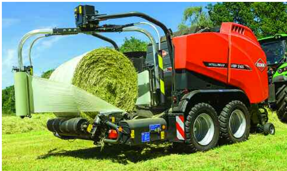
Kuhn's new VBP 3165 now features a twin-reel film binding system like that of the brand's fixed chamber balers.
