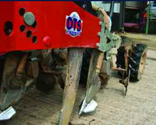
The DTS comprises a straight disc which cuts trash and initiates the rip line for the ensuing leg.
