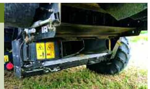
A Redekop SCU, fitted here to a Case IH 7230 combine, achieved an 83% reduction in meadow brome seedlings in the following crop in a 2021 trial.
