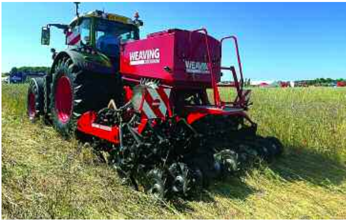
The Weaving GD is available as a mounted or trailed drill and is a low disturbance machine.
