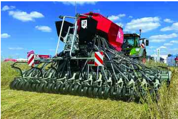
The Novag T-ForcePlus is a hybrid drill that has a disc and tine working together.
