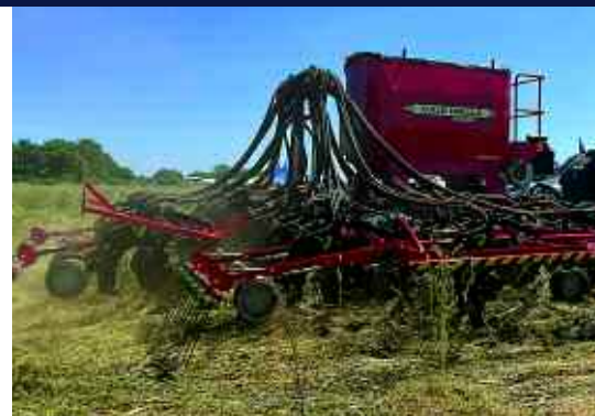
The range of Dale Drills are designed to allow farmers to direct drill or sow into min-till and conventional seedbeds.
