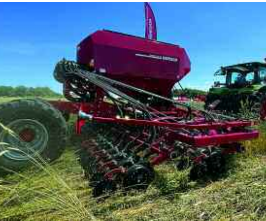
Horsch has a specially designed single disc coulters for the Avatar.
