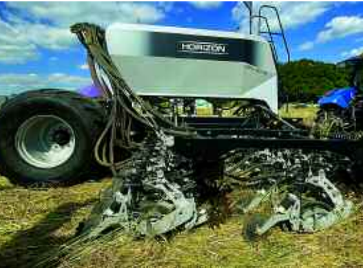
The Horizon DSX has been designed as a modular drill that starts as a 4m drill which can be extended with optional modules.
