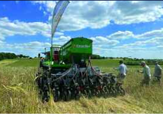
The Cross Slot drill is designed not to block in crop residues and minimise soil disturbance.
