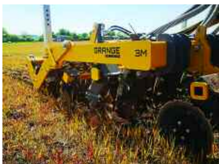
A key feature of the cultivator is Grange’s low disturbance leg and rear cultivation system to aid in the soil loosening process.
