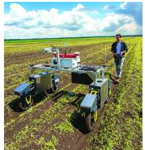
The TuberScan system comprises of radar, GPS units and an in-field camera that surveys the field throughout the growing season.
