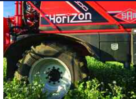
Continental's ContiPressureCheck monitors the pressure and temperature of tyres using sensors in the tyre.
