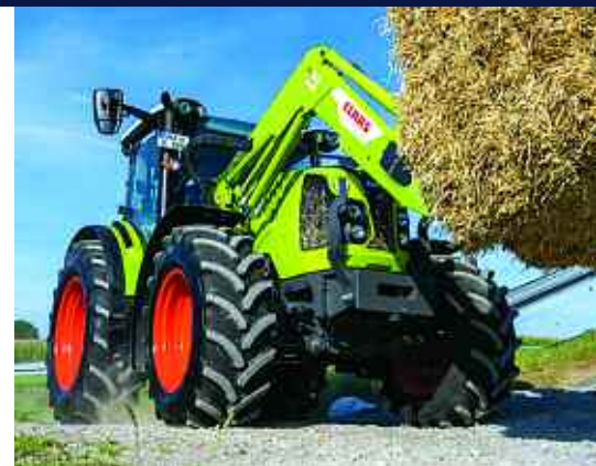
The new Vredestein Traxion 70 features curved lugs and a large contact area in the middle of the tread.
