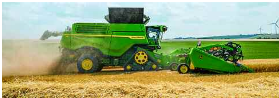
Powering the X9’s performance is a new 13.6 litre six-cylinder engine, capable of delivering up to 700hp, which enables combines to run for 14 hours without needing to refuel.
