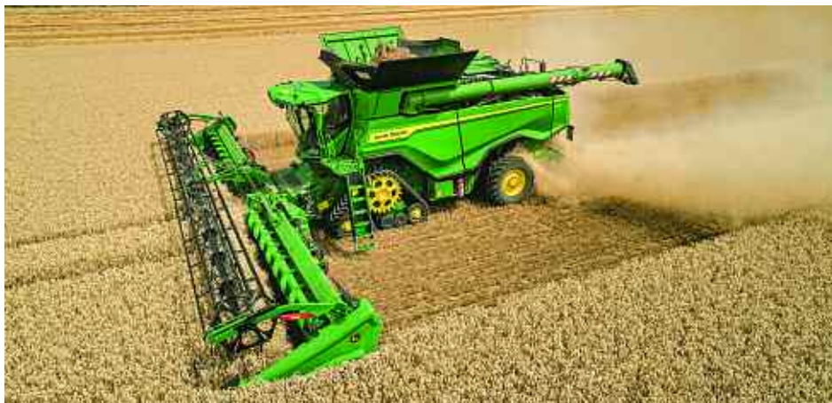
It's the X9's capacity which makes it stand out from the competition, with X9 1100 capable of harvesting wheat at 100t/hour at less than 1% grain loss.
