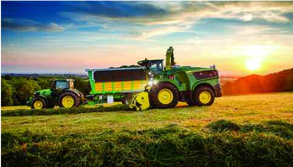
The 9000 Series are now equipped with a newly designed discharge chute, which is 20cm longer than the previous version.
