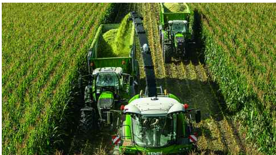
Fendt's Katana 850 has an in-line six-cylinder engine from Liebherr, a displacement of 18 litres, and an output of 847hp/623 kW.
