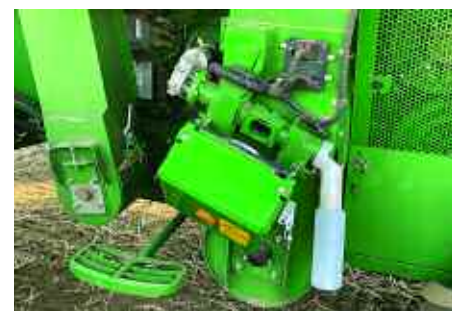
Data collected by HarvestLab can produce yield maps to help farmers identify where in the field crops are getting the right level of nitrogen.
