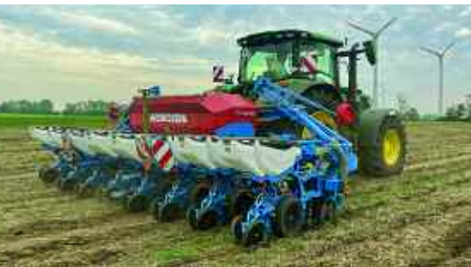
Autopath will adjust the position of the drill to precisely follow the lines of slurry.
