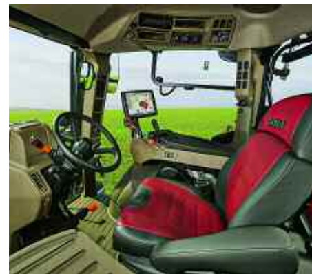
In-cab upgrades to the Case IH Puma include a phone mount, USB power ports and a tablet mount to ease in-cab management.
