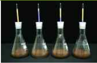
Volatilisation can be demonstrated using Dräger tubes - these contain yellow crystals which turn blue when ammonia is released.
