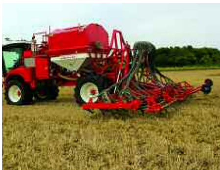
Fitting the Bateman platform with Weaving Sabre Tine coulters gives much more direct drilling flexibility at Manor Farm, especially where trash levels are high.
