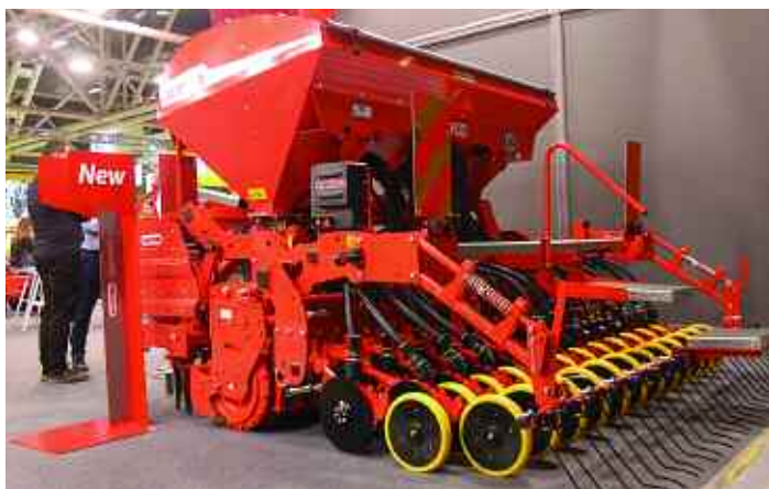
Maschio Gaspardo's Alitalia combination drill now features upgrades including a redesigned hopper and external distribution heads.
