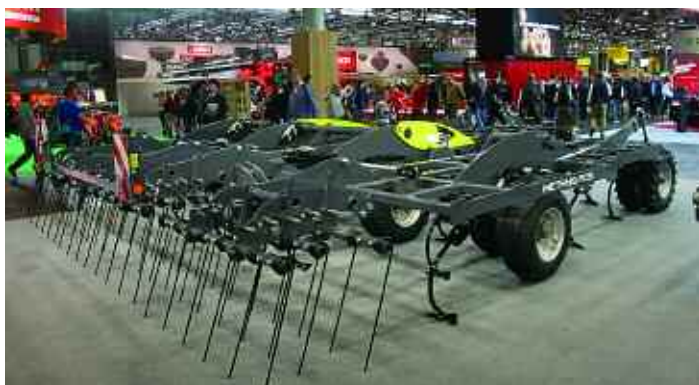
Sky's Methys PCS shallow cultivator is designed for slicing through root matter at depths of around around 5cm (2in). A 6m unit features 29 A-share-equipped tines set across seven rows.
