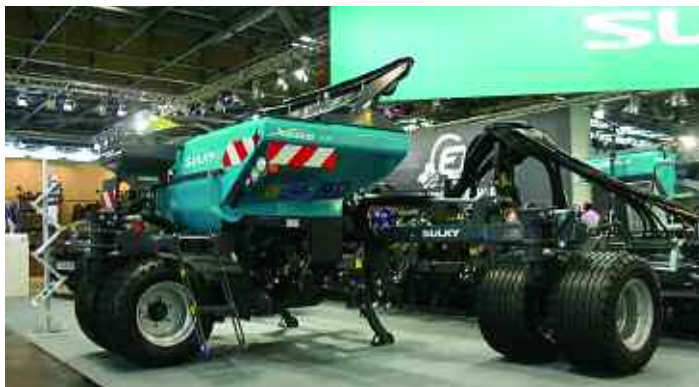
Sulky's prototype press wheels extend hydraulically out beyond the tractor to consolidate the soil ahead of the outer reaches of the drill behind.
