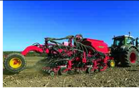
The Proceed is a prototype drill from Väderstad, aimed at fine-tuning seed placement.
