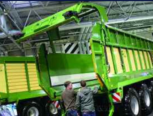
Krone's GX self-unloading trailer has applications in root crops and vegetables, as well as maize and even combinable crops.
