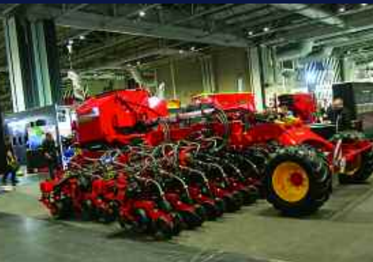
Still undergoing development trials and likely to be heavily revised before a launch, Vaderstad's Proceed hybrid drill uses many components from the Tempo precision seeder.
