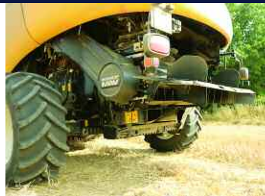
The chaff stream is separated from the straw and passes from the sieves into the SCU that's fitted below the straw chopper.
