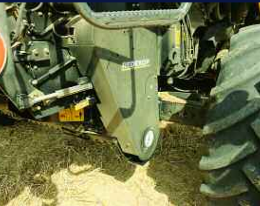
The drive for the low-slung unit comes to the side, so the axle had to be widened to 3.8m to accommodate it.
