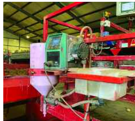
A direct injection system feeds a Team Sprayer CTC2 hooded canopy with twin rotating nozzles, enabling all seed to be accurately treated in-house at Pryor & Sons.
