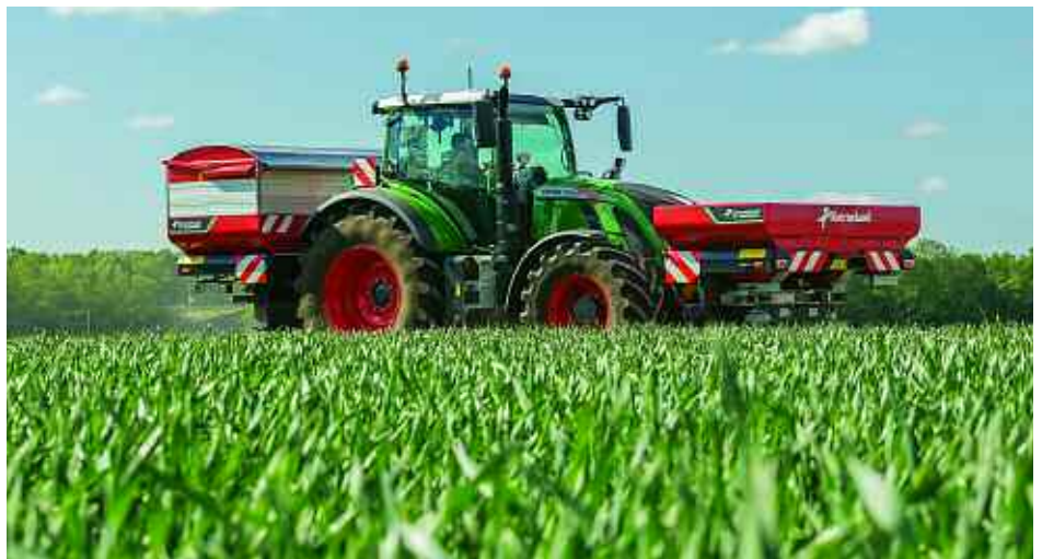
Kverneland’s weigh cell equipped Exacta models can now be used in a front- and rear-mounted disc spreader combination.
