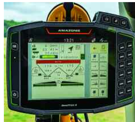
One of Amazone's latest precision additions to its spreaders is WindControl which senses the direction and strength of the wind.
