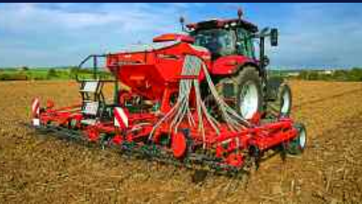
Kuhn's new Megant 602R drill is lightweight allowing for it to be operated by tractors with as little as 150hp.
