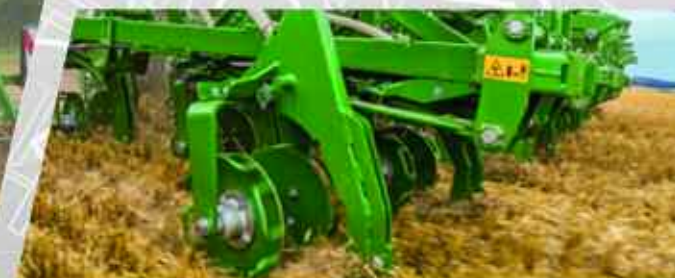
Each individual hard-faced chisel opener is guided at the perfect planting depth by the following Reflex rollers.
