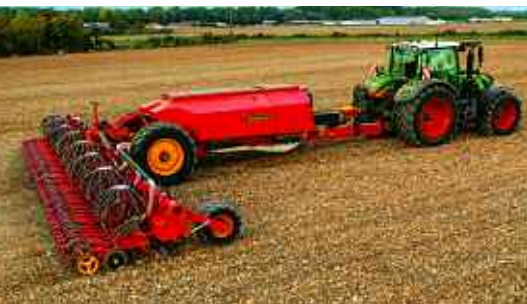
Väderstad's Inspire is a new 12m, high-capacity precision seed drill with a responsive double disc seed coulter system.
