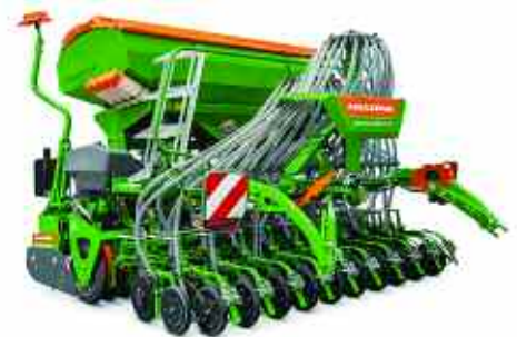
The key feature of Amazone's Centaya-C pneumatic harrow-mounted drill is its 2000-litre twin chamber hopper.
