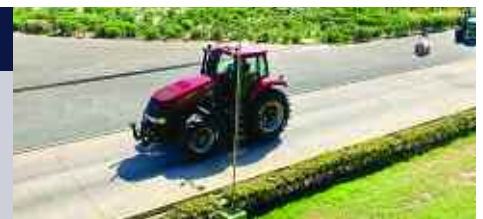
BKT has the Indian ag tyre industry's only 'real world' external test tracks, including tarmac to assess road characteristics, a tarmac/mud/stone combination for durability tests, and an automated track.
