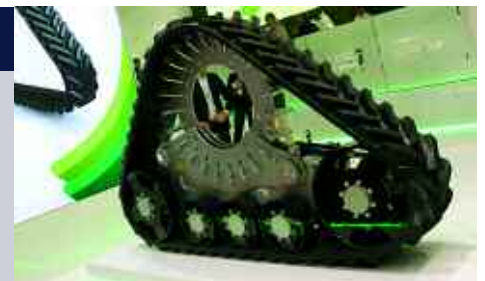
Track production at Bhuj recently began, with current production at 20-25/day of the 18x6x44 units in a pre-production/testing phase.
