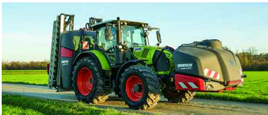
Horsch's Leed FT is an intelligent spraying technology which is front-mounted on a three-point linkage and offers additional spraying capacity.
