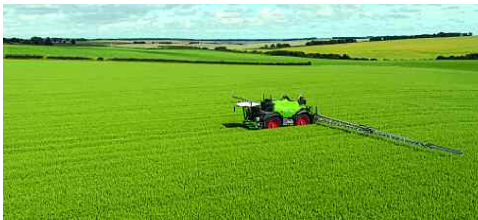
The Rogator can now have six OptiSonic boom height sensors to improve application accuracy.
