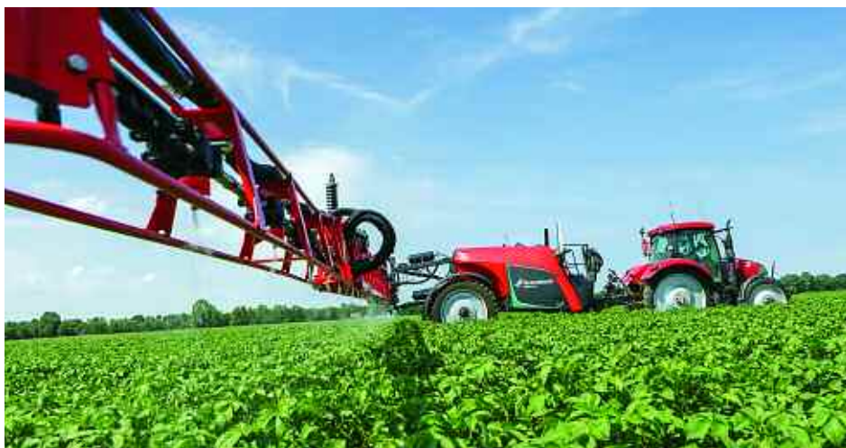
A new optional feature of Kverneland's sprayer range is SpotSpray technology, which is an extension of variable rate application maps.
