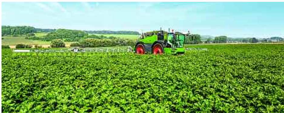
Fendt's ContiRinse system aims to make switching between different chemicals quicker as it begins the rinsing cycle during spraying.
