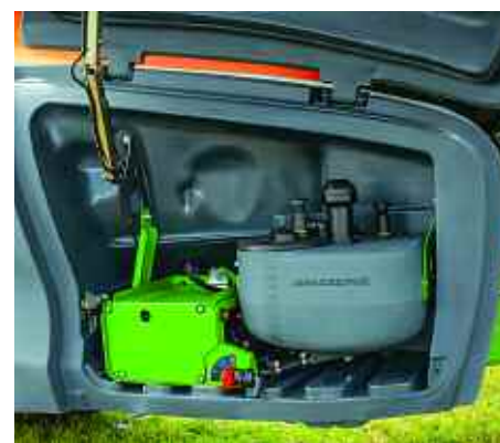
DirectInject is a new system that has been designed to be integrated into the spray circuit of Amazone's UX01 Super sprayers.
