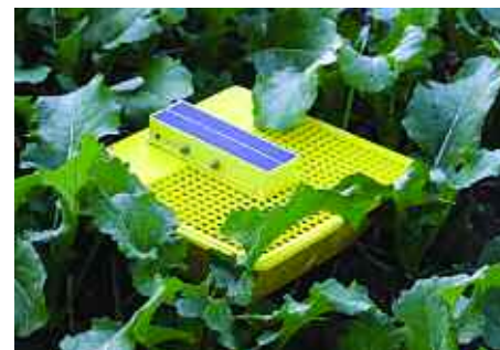
MagicTrap is a new pest monitoring solution that enables farmers to detect and assess cabbage stem flea beetle in oilseed rape crops.
