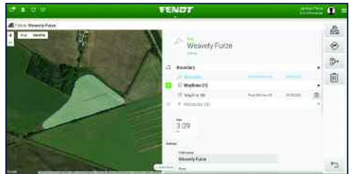
Waylines are saved to FendtONE and then shared between different machines and operators.
