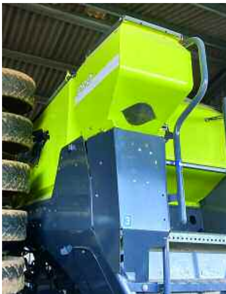
Specifying the additional 120-litre Pro Hopper allows companion crops or slug pellets to be applied in the same pass as the primary crop.
