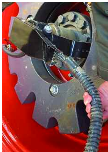
Claas has invested in the manufacturing of its Central Tyre Inflation Control system, having taken a controlling interest in the maker.
