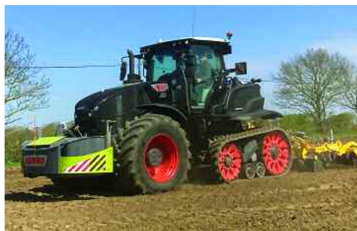
For users seeking even greater ground contact, Axion 930 and 960 tractors are available with Terra Trac rear tracks, which can be supplemented with a CTIC system on the front axle.
