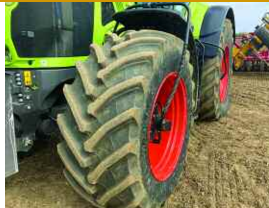
Claas says customers keen to maximise soil protection without compromising road comfort are increasingly specifying its CTIC (Central Tyre Inflation Control) system on larger Axion tractors.
