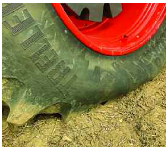
The primary benefit of variable tyre pressure systems is that they lengthen the contact patch of each tyre, with negligible effect on transport width of just a few additional millimetres.
