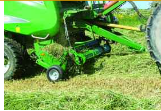
The farm's V6 760 features McHale's 2.1m five-bar pick-up, which feeds the 15-knife chopping unit for the 1500 silage bales made annually.
