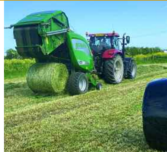
Via the ISOBUS controller or compatible tractor terminal, the V6 760’s three-belt variable chamber can be adjusted to produce bales from 0.70-1.68m diameter.
