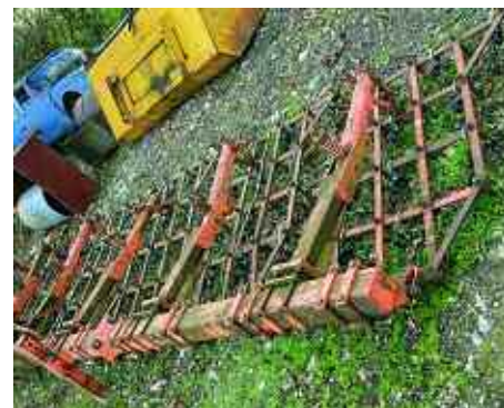
Andrew built his own straw harrow from a second-hand frame and new tines to lightly scratch the surface and distribute chopped material.
