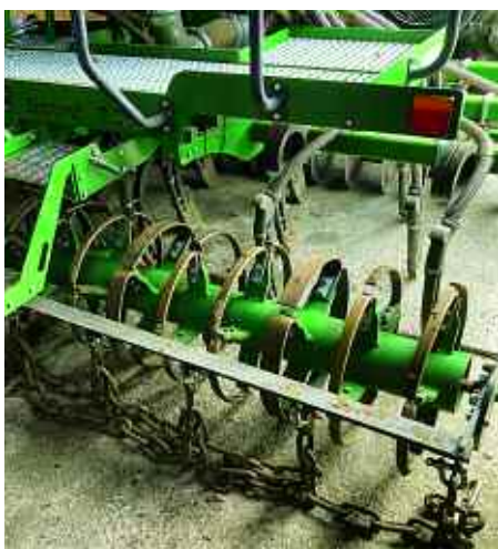
The press rings and following chains are reckoned to be simple and effective, filling the slots with soil without compressing them closed.
