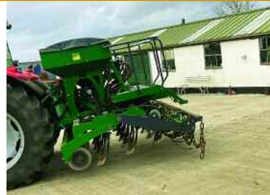
The Simtech T-Sem's tine coulters are staggered over three rows, which has been found to do a good job aiding trash flow.
