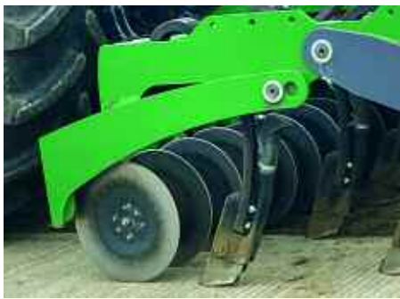
Each seeding row on the Simtech T-Sem begins with a straight disc that slices an opening for the following inverted T-shaped seeding boot.
